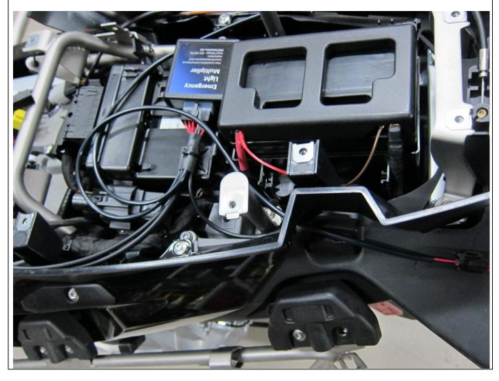
Secure the ELM module to the carrier of the GMSF with the Velcro provided. Note that there is a tab on the right side of the GMSF mount – make sure the ELM module sits flat on the carrier.
