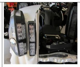
This is what the finished installation will look like. Follow the notes below for tips on the installation. **Note:** The blue duplex light connection has been replaced with a cable running to the rear light pod to connect directly at the flasher board.
